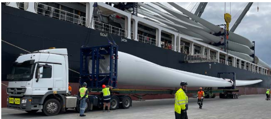
Turbine blade being unloaded at Napier Port.
